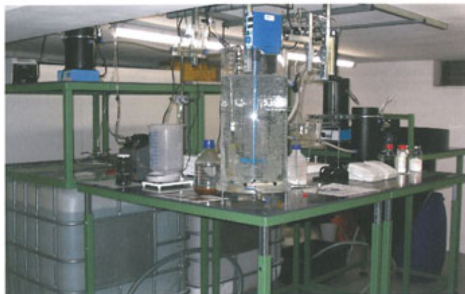
TEST PLANT EXPERIMENT: Mine water treatment plant at GFI GmbH, Dresden Image 3
